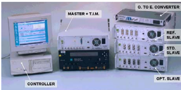
Figure 8 : parts of the timing system
